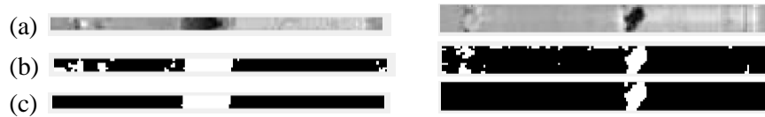
Fig. 7. Process to find the column indexes of the defects. (a) Image blocks cropped from the sparse image E (image blocks in red rectangles, Fig. 6(b)). (b) Image block binarization results. (c) Results obtained by keeping the maximal-connected component.
