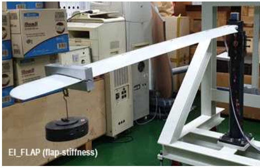
a) Flap stiffness measurement
