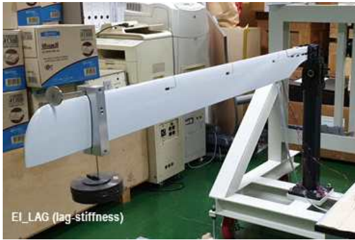
b) Lag stiffness measurement
