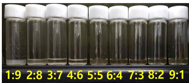
Figure 2. From left to right, the yellow number indicates the ratio of HFIP to TFA. \alpha -chitin (from Sigma-Aldrich Co., Ltd.) powders were not dissolved when they were added in HFIP-TFA binary solutions ranging from 1:9 to 6:4. It was confirmed to be completely soluble in the ratio of 7:3 to 9:1.
