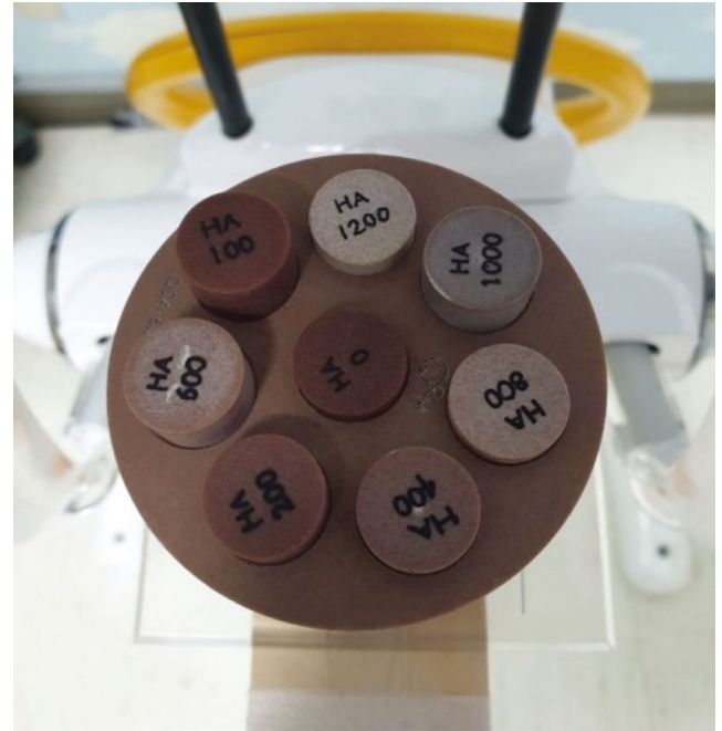
Fig. 2. The phantoms available for use in this study. Of these, HA0, HA400, HA800, HA1000, and HA1200 are used.
