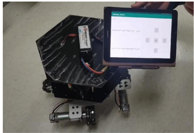
Fig. 10. Balancing control error measuring equipment by wireless communication of ball robot.
