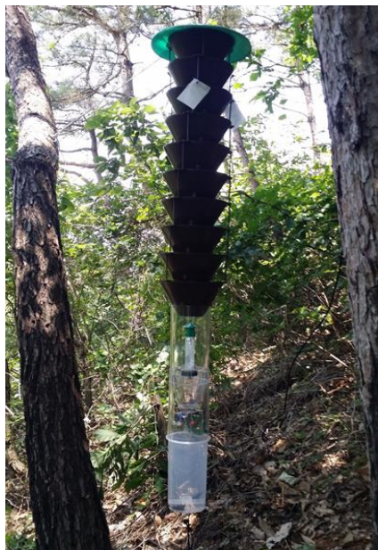
Fig. 2. Smart trap for pine-wilt disease control
