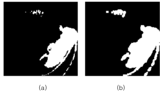
Fig. 9. Dilation operation using insect image
