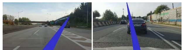
Fig. 24. Lane detection failure image visualization
