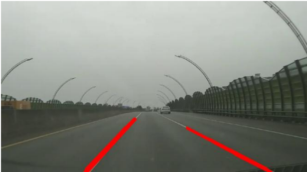
Fig. 11. Example of proposed lane detection method result
