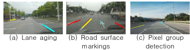
Fig. 13. Lane detection failure result
