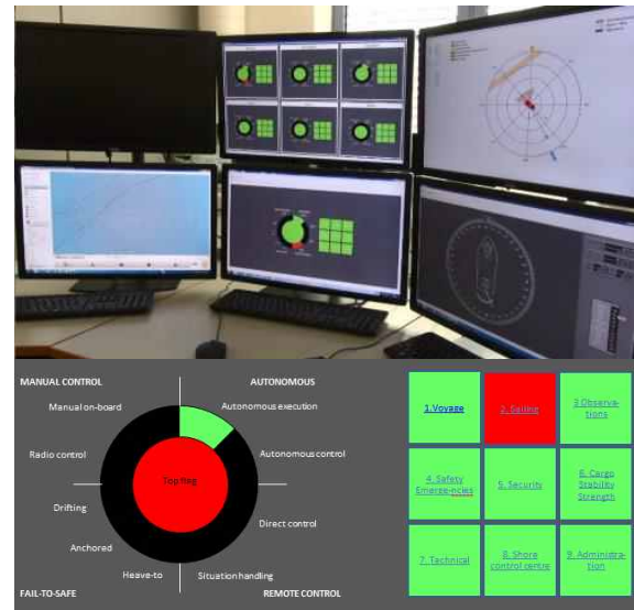
Fig. 3 Operator's workstation and dashboard to display information of shore control center in MUNIN Project
