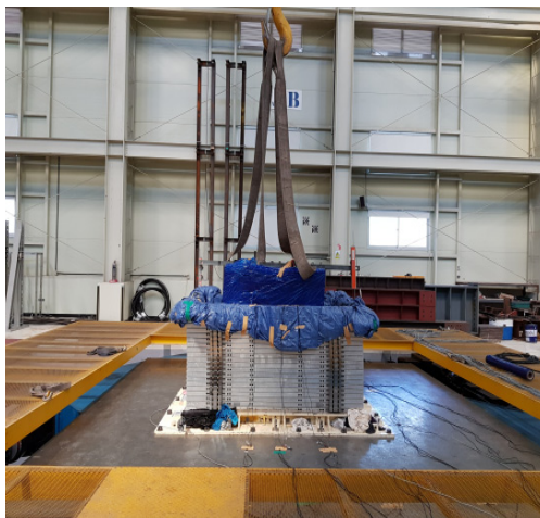
(a) Lamina Box on the Shaking Table
