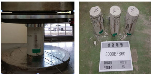
(a) Compressive strength test (b) Failure condition after test
