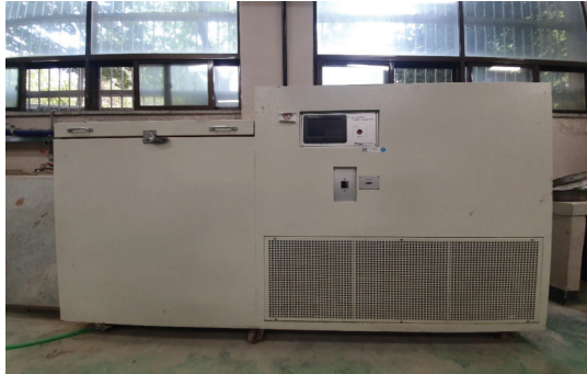
Fig. 3. Freezing-thawing apparatus in the test
