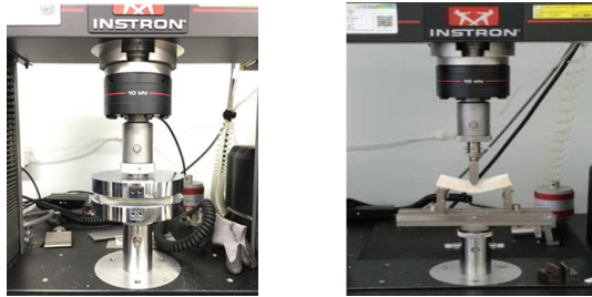
Fig. 5. Destruction mechanism for compressive and bending strength measurement
