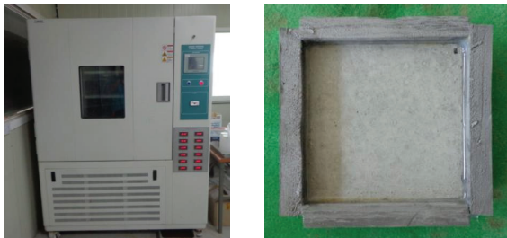
Fig. 4. Scaling resistance test
