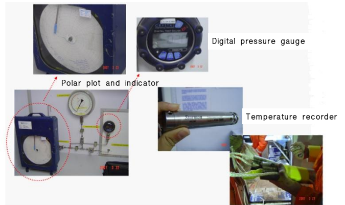
Fig. 3. Measuring system of hydrotesting.
