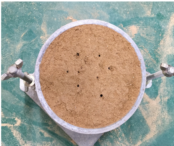
Fig. 9. Upper view of compaction mold after penetration test
