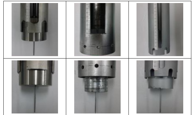
Fig. 3. Penetration steel wire and measuring rules
