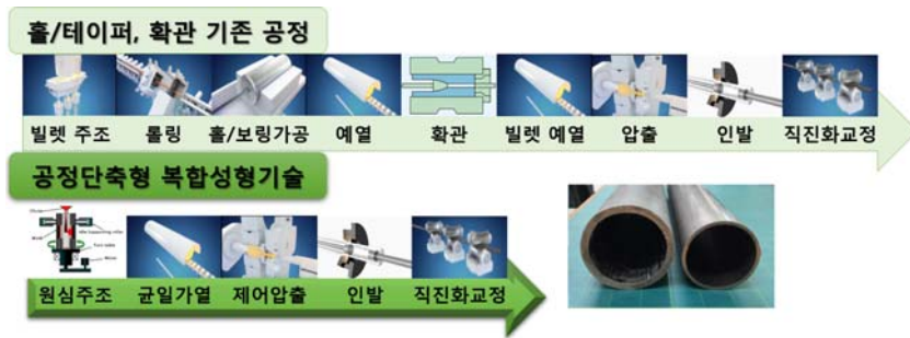
Fig. 6. Schematic diagram of new seamless tube manufacturing process.
