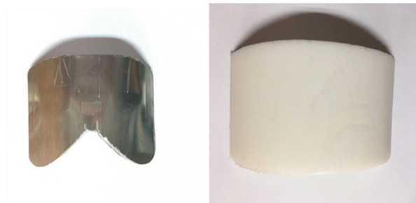
(a)Aluminum 7.3mm (b)Silicone 21.5mm Fig. 1. Manufactured shield.
