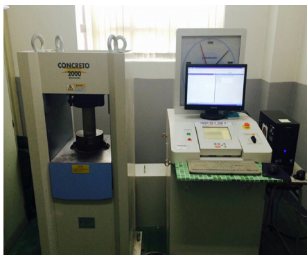
Fig. 6. Uniaxial direct compressive test machine
