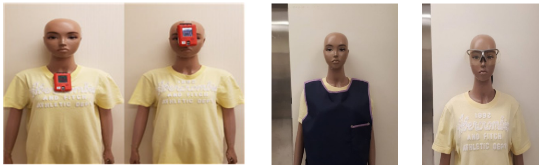
Fig. 7. Specific location of pocket dosimeter position in the phantom
