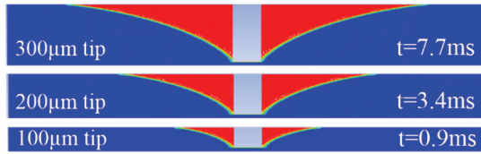
Fig. 8. Simulation results of solution distribution near the \mu -tip for different \mu -tip length.
