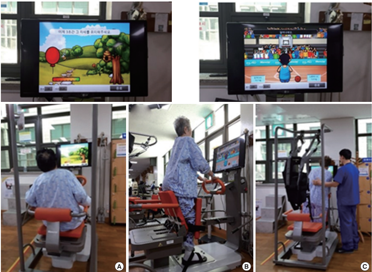
Figure 1. Trunk control rehabilitation robot training. A: weight shifting sitting, B: sit to stand, C: weight shifting standing
