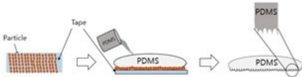
Figure 2. Schematic steps to prepare a micro- and nano-structured PDMS film.
