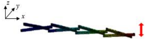
Fig. 13. The 1st mode shape of 1-stage scissors structure
