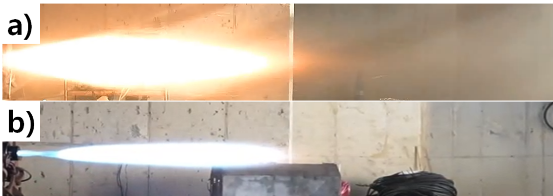
Fig. 7 Test motor plumes with HTPB/AP/AL propellant (a) and ETPE/RDX propellant (b).
