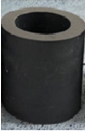
Fig. 4 Energetic thermoplastic propellant grain.
