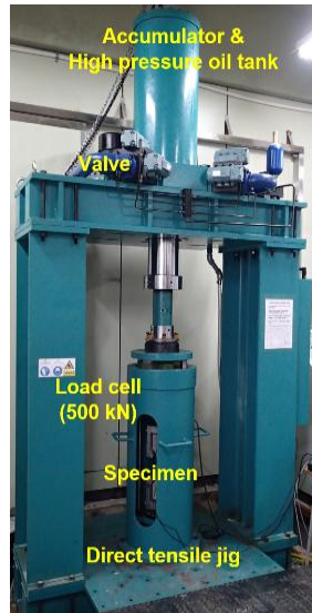
Figure 4. Dynamic direct-tensile test equipment
