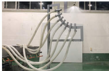
Fig. 4. Test of spray angle of deflector
