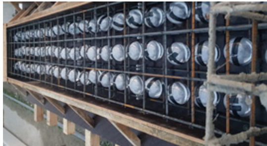
Fig. 2. Production of Hollow core Specimen with Liquid
