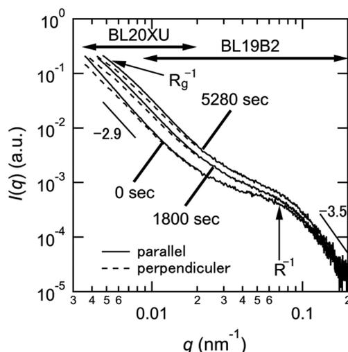
**Figure 1.** The scattering profile combined BL20XU and BL19B2 data is plotted as a function of  $q$  at 0 sec, 1800 sec and 5280 sec after the start of shearing.
