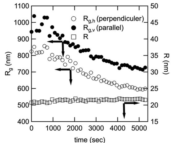
**Figure 2.** The size of agglomerate in the direction of perpendicular and parallel to the shear flow and the size of aggregate with time.
