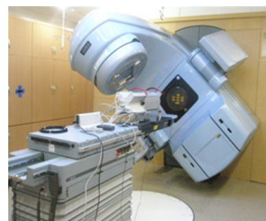
Fig. 1. The phantom setup for verification on Clinac IX
