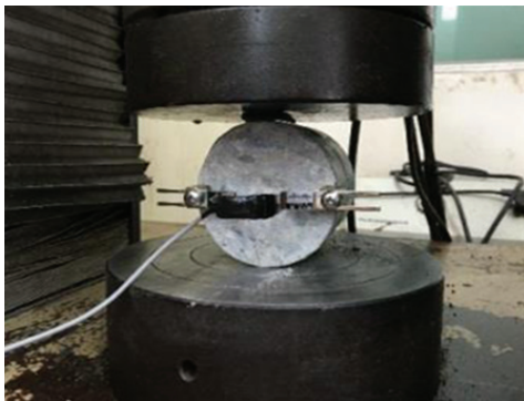
Fig. 1. Loading for crack inducing and measuring
