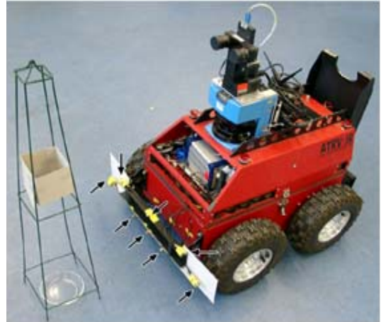
Fig. 1. Gas tracker robot developed in Univ. of Tübingen [5]
