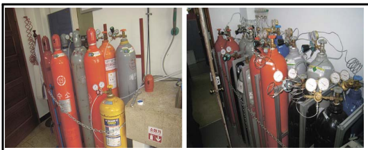
Fig. 2. Poor management of gas cylinders in University Lab[1].
