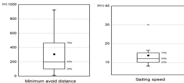
Fig. 4. Survey result on minimum avoid distance and sailing speed.
