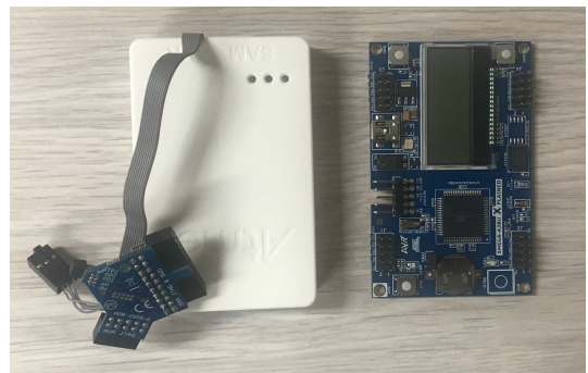
Fig. 5. In-circuit debugger; Atmel Ice & XMEGA-A3BU Xplained
