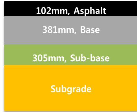
Fig. 4. Asphalt pavement structure used in the analysis
