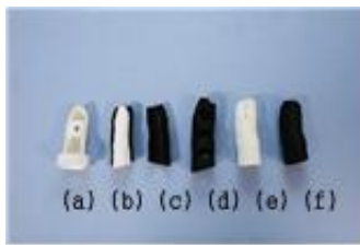
Fig. 9. 3D printer finger brace (a) stack splint (b) splint under (c) splint on (d) hole design (e)(f) stright design.
