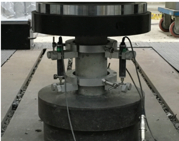
Fig. 1 Test of compressive strength and elastic modulus
