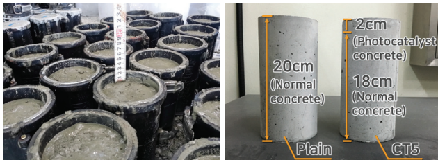
Fig. 3 Concept of separated casting on the photocatalyst concrete
