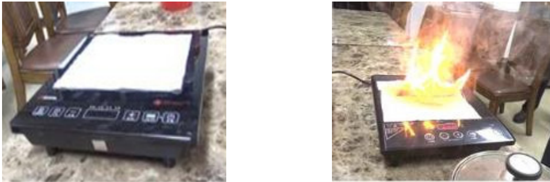
Fig. 8. Kitchen towel Combustion in Highlight Electric Range
