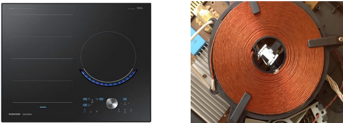
Fig. 4. Structure of Induction Electric Range (newspim, naver blog)
