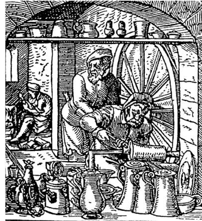
Fig. 4 Wooden spinning lathe with a manually operated flywheel to spin the workpiece [3]
