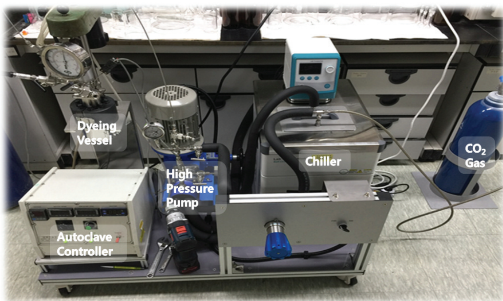
Figure 1. Supercritical CO 2 dyeing equipment.
