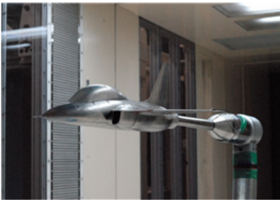
Fig. 1. KTX-2 Model for wind tunnel testing
