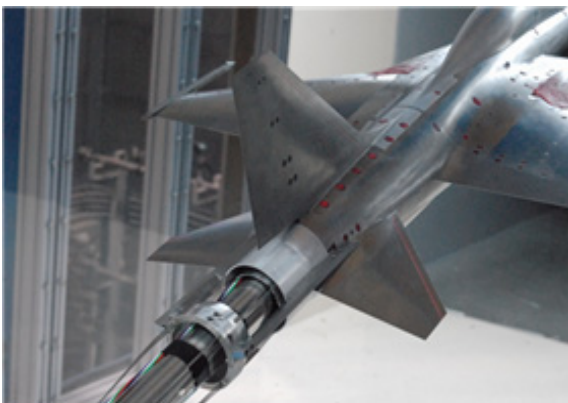
Fig. 2. Internal drag measuring rake installed at the rear of model
