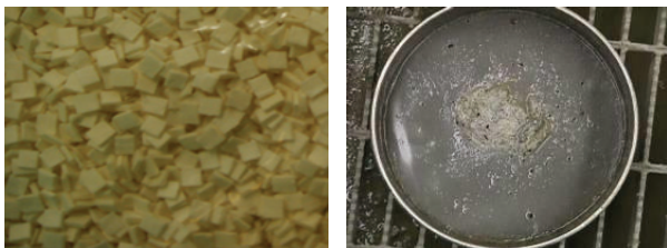
(a) Chip typed CF (b) Residual CF through sieve
