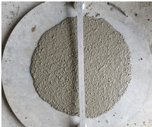
Fig. 4. Effect of the unit binder on slump flow values
