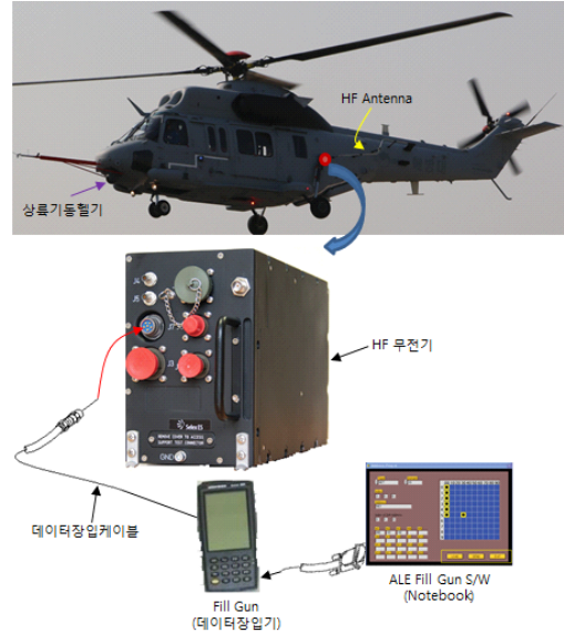
Fig. 2 Cable Connection for Data Loading to HF Radio
