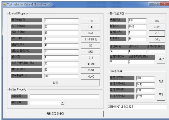
Fig. 4 Optimal cutting tool rotational speed and feed rate of vertical CNC milling calculated by CATIA V5 tool maker program
