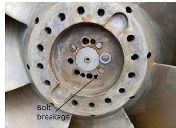
Fig. 18 Photograph of bolt breakage
