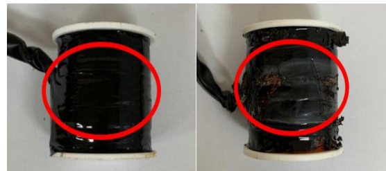
(a) Before failure (b) After failure Fig. 1 Photos of before and after fuel pump failure
