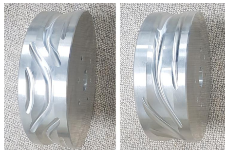
(b) Machined ball gear cam
