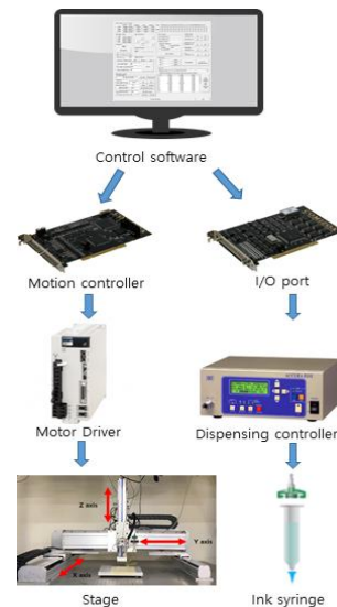
Fig. 1 Sensor manufacturing system
