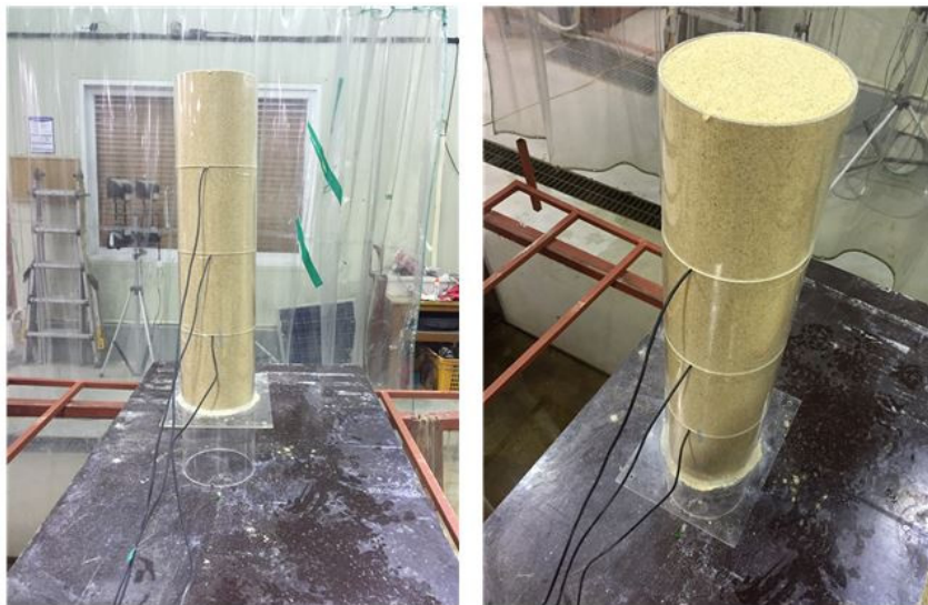
Fig. 8. Complete tensiometer installation
