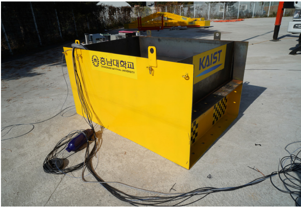
Fig. 3 Floating body for underwater shock experiments
